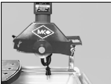
(A) Loosen the Blade Guard Retaining Wingnut
