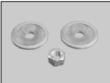
(A) Remove and clean the Inner and Outer Flanges and the Blade Retaining Nut
