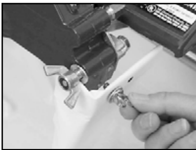
(A) Remove Thumbscrew and washer from back of Blade Guard
