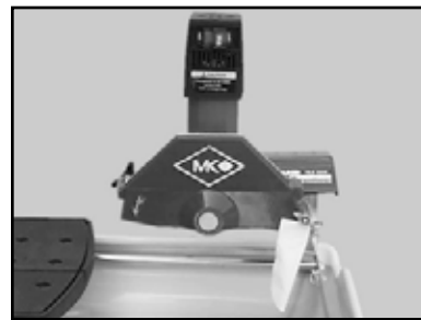
(B) Install the Thumbscrew through the Washer and Splashguard then align to the hole found on back of the Blade Guard and tighten
