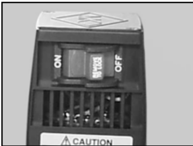
(A) Locate the Lockout Pin in the center of the ON/OFF Switch toggle (the Lockout Pin has "Remove To Lock" highlighted)
