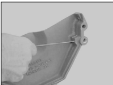
(G) Rod Cooling Channels and recheck flow
