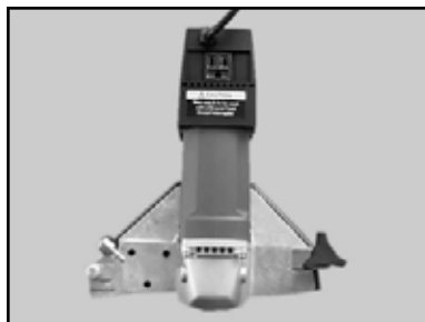
(B) Loosen the Blade Guard Retaining Knob and open the Blade Guard
