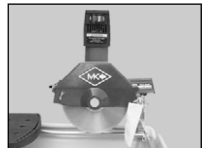
(C) Inspect the Diamond Blade for damage – verify the blade is correct for the type of material being cut
