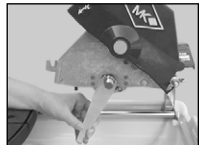
(C) Place the Shaft Wrench on the Motor Shaft (NOTE: the Outer and Inner Flanges and the Blade Nut are removed in the photo above) rotate blade shaft so shaft wrench is engaged.
