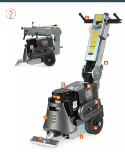
The Gladiator removes the worst of today's hard and soft goods, such as ceramic tile, wood floors, thin-set, sheet vinyl, linoleum, and more. Its compact design makes it ideal for use in confined spaces, while the side slide weights add extra head pressure when forward and improved traction when moved over the back wheels.
