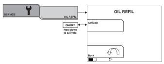
The gauge shows the oil level in percentage with even tens. Hold the selection key down to refill oil. The pump will shut off automatically when the tank is full.
