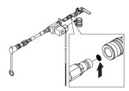
Daily inspect the nipple coupling mesh filter, clean when needed.
