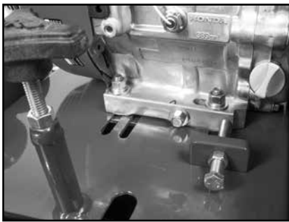
(L) Tighten the Engine Mounting Bolts.
