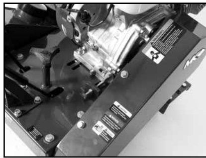
(M) Install the Belt Guard and Belt Guard Retaining Bolts.
