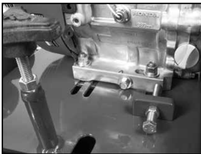
(D) Locate the four upper Engine Mounting Nuts on both ends of the motor and loosen.
