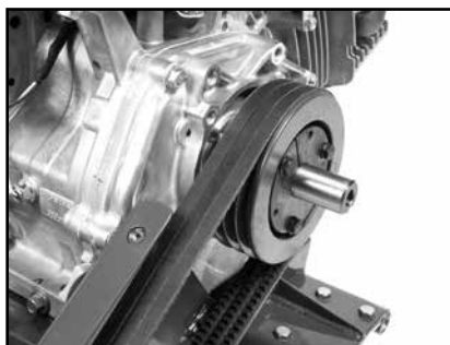
(G) Remove the old belts from the Engine and Blade Shaft Pulleys.
