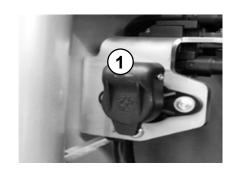
Insert plug (1) into the charging socket.
