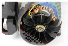
Separate cooling of the electric motor and compressor allows for continuous duty and a long life.
