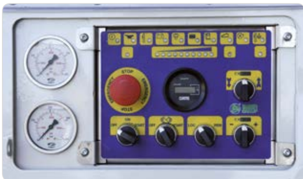
Antivibration control panel with electromechanical controls
