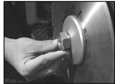
(O) Verify the Blade Retaining Nut is seated in the Outer Flange
