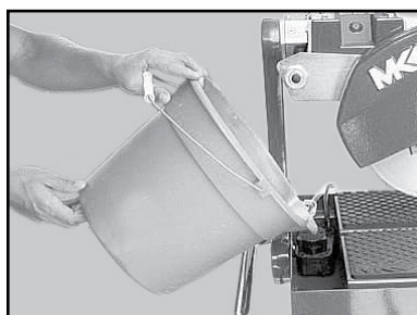
(B) Fill the Water Basin until water completely covers the Water Pump suction.
