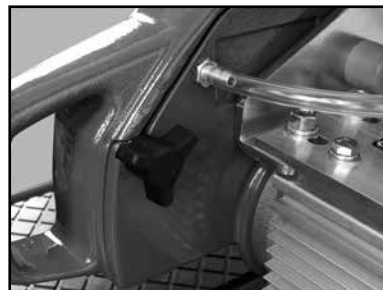
(Q) Tighten the Blade Guard Retaining Knob.
