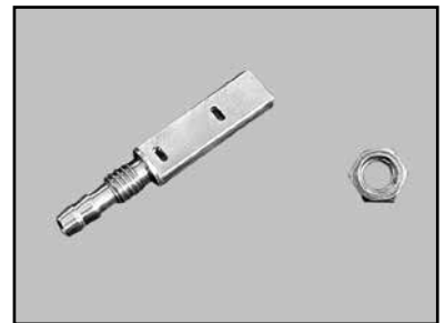
(F) Rod (clean out) the Cooling Manifold and then recheck flow.
