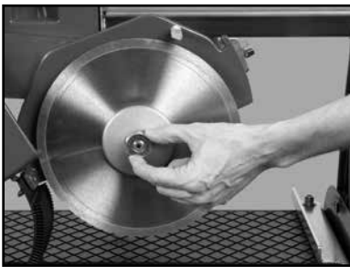
(M) Install the Blade Retaining Nut.
