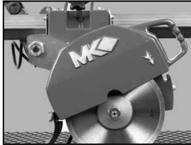
(K) Verify the Directional Arrow of the Blade matches the Directional Arrow of the Blade Guard.
