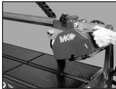
(E) Raise Cutting Head. Retighten Cutting Head Height Lock.
