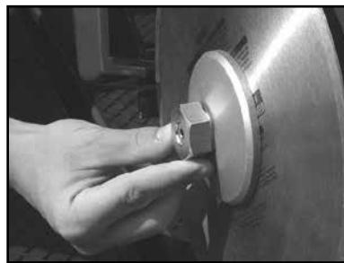
(N) Verify the Blade Retaining Nut is seated in the Outer Flange.
