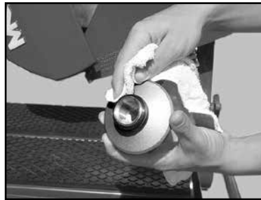
(B) Clean the Inner Flange.
