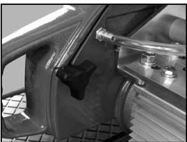
(G) Loosen the Blade Guard Retaining Knob.
