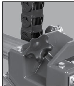
(H) Tighten the Cutting Head Locking Knob.
