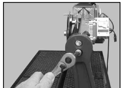
(F) Loosen the four Guide Rail Adjusting Screws using a 1/2-inch socket.
