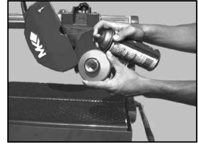
(C) Lubricate the Inner Flange Gasket.
