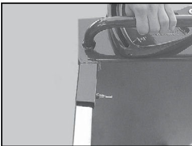
(D) Lift the end opposite of the cutting head; align the Leg with the Retaining Slot on the saw and install the Leg.
