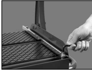
(B) Remove the Back Stop.
