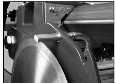
(C) Run the saw until clear water is seen at the blade cooling ports (Approx. 1 minute).
