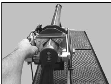
(G) Adjust the Guide Rail until it is aligned both vertically and horizontally.
