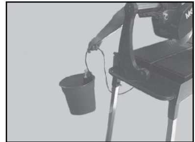
(C) Place the Water Pump in an external container.
