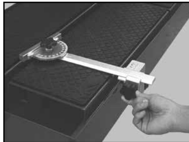
(B) Place the Protractor on the side of the cutting table. Adjust the Protractor to fit the tile being cut and tighten the Retaining Knobs to lock the Protractor.
