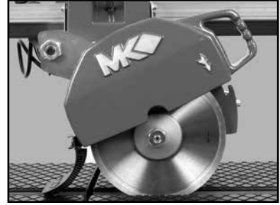
(L) Verify the Directional Arrow of the Blade matches the Directional Arrow of the Blade Guard
