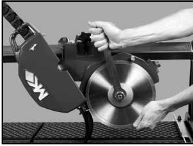
(A) Remove the Diamond Blade and Inner Flange.
