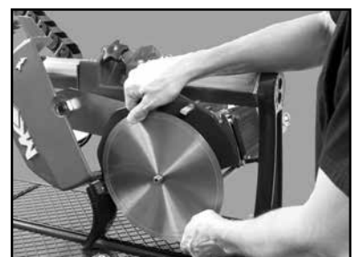
(I) Remove the old Diamond Blade.
