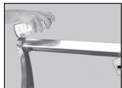
(C) Lubricate the Guide Rail.
