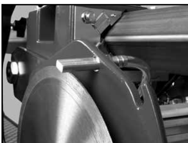
(G) Verify proper cooling flow on both sides of the blade.
