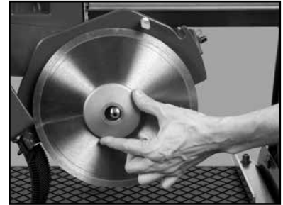
(L) Install the Outer Flange.
