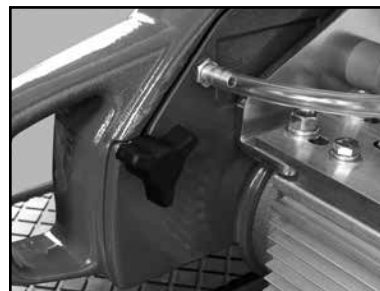
(E) Loosen the Blade Guard Retaining Knob.
