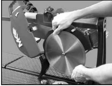
(K) Install Diamond Blade onto Blade Shaft
