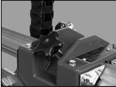
(A) Loosen the Cutting Head Locking Knob.
