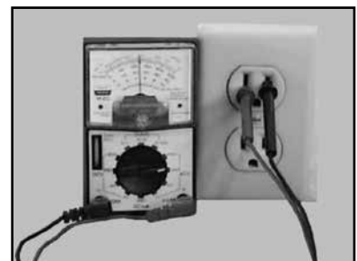
(F) Check power source voltage is 115v – if not 115v, move to another circuit.
