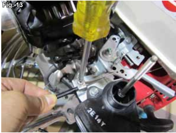
Step 10: Secure the wire to the cable clamp while pushing with slight pressure forward. (Fig. 13)
