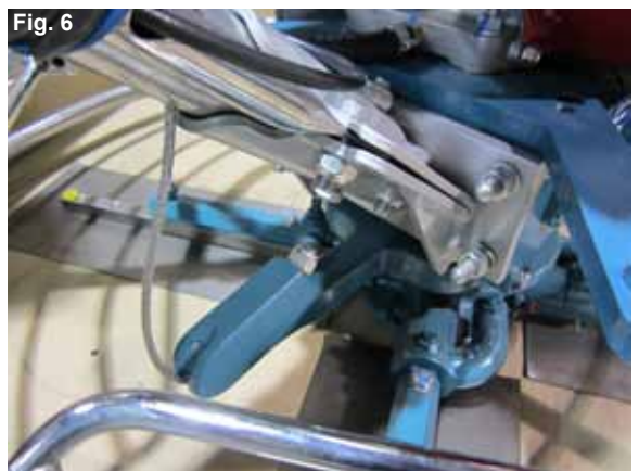
Step 4: Lift and install handle to position using the supplied four sets of lockwashers and nuts. Do not torque greater than 18ft-lb. At the yoke; tighten the locknut for pitch control cable (Fig. 6). If the cable is too loose or tight, the pitch control range position can be moved by changing the position of the stop screw (Fig. 5). The factory default is the middle position. Turn the pitch control knob completely clockwise and check for maximum pitch possible. This is possible when the clearance between the yoke and underside of the gearbox is enough to pass a business card through.
