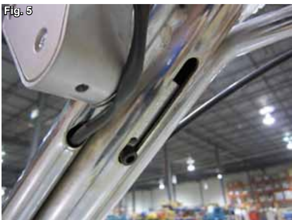
Step 4: Lift and install handle to position using the supplied four sets of lockwashers and nuts. Do not torque greater than 18ft-lb. At the yoke; tighten the locknut for pitch control cable (Fig. 6). If the cable is too loose or tight, the pitch control range position can be moved by changing the position of the stop screw (Fig. 5). The factory default is the middle position. Turn the pitch control knob completely clockwise and check for maximum pitch possible. This is possible when the clearance between the yoke and underside of the gearbox is enough to pass a business card through.
