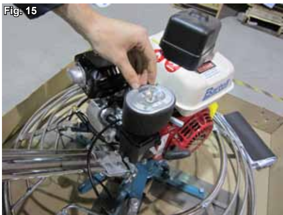
Step 12: Reinstall air filter and cover (Fig. 15)
