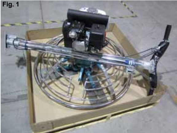
Step 1: Trowel shown with handle separate. (Fig. 1)
