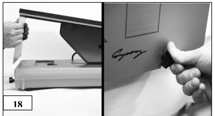
18 Set Saw Assembly on top of the Water Bath and tighten Thumb Screws (4).
