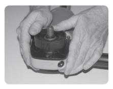
3. Place spacer over grinder head with the ExteriorGroove (A) facing down, toward the grinder head.Push down until InteriorO-ring (B) snaps into place.
