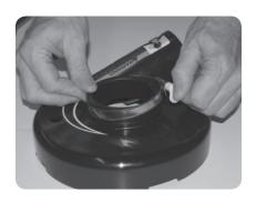
**4.** Take shroud clamp and place on the top of the shroud loosely.
