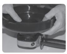
5. Place shroud on grinder, push and twist until Shroud Interior O-ring (C) snaps into Spacer Exterior Groove (A). (For Bosch model grinders, Shroud Interior O-ring (C) snaps directly onto grinder head.)
