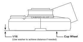
Shim is for use with a DeWalt or Jepson grinder, or as cup wheel is worn, it may be used to achieve distance if needed.
