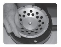
Once shroud is tightly attached to the grinder, attach grinding wheel as normal. Ensure cup wheel does not contact shroud.
