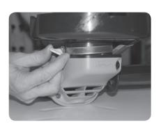
**6.** Tighten clamp with wing nut so it is firmly attached to grinder head.
