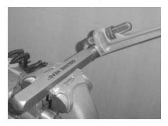
2) Pull the eccentric rotor assembly out of the housing. (If the bearings are stuck and you have difficulty removing them from the housing, screw end cap partly back into the housing and bounce the head and cap down on a block of wood, in order to loosen the bearings from their seat, then pull out rotor assembly.)
