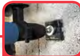
Square off using the rapid action Square cutter in softer materials
