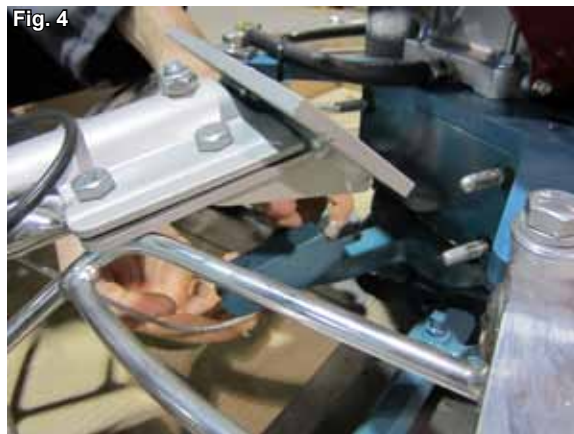
Step 3: Install pitch control cable to yoke and install locknut loosely (Fig. 4). If needed, turn pitch control knob counter-clockwise until the stop screw is at the lowest position (Fig. 5).
