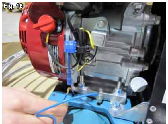
Step 13: Route engine safety shut-off wire around engine and install. There are two types that may be available with the machines. (Fig. 16 and 17)
