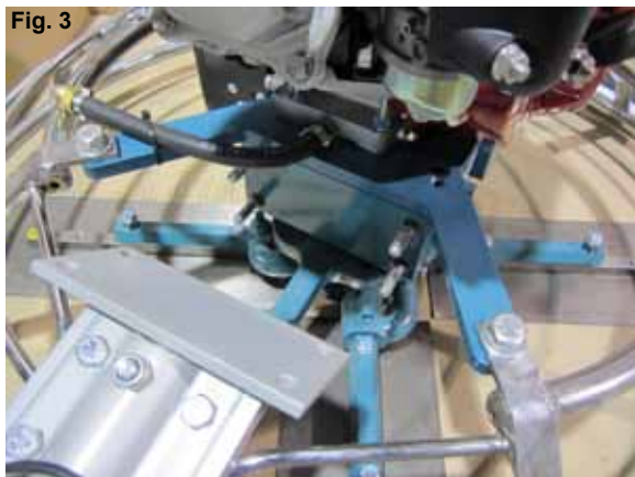
Step 3: Install pitch control cable to yoke and install locknut loosely (Fig. 4). If needed, turn pitch control knob counter-clockwise until the stop screw is at the lowest position (Fig. 5).
