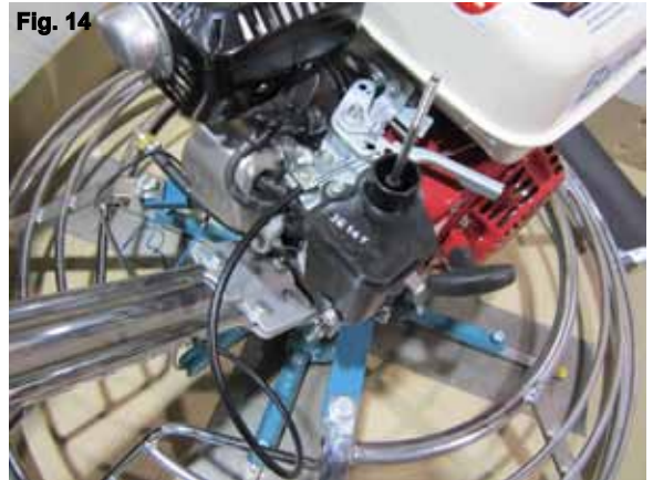
Step 11: Check operation of throttle control lever. (Fig. 11 and 14)
