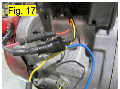
Step 13: Route engine safety shut-off wire around engine and install. There are two types that may be available with the machines. (Fig. 16 and 17)
