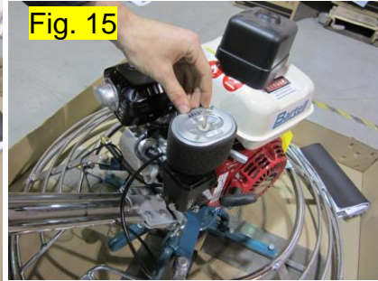
Step 12: Reinstall air filter and cover (Fig. 15)
