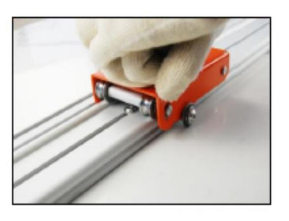
Make one continuous motion scoring on the tile with the guide car.
