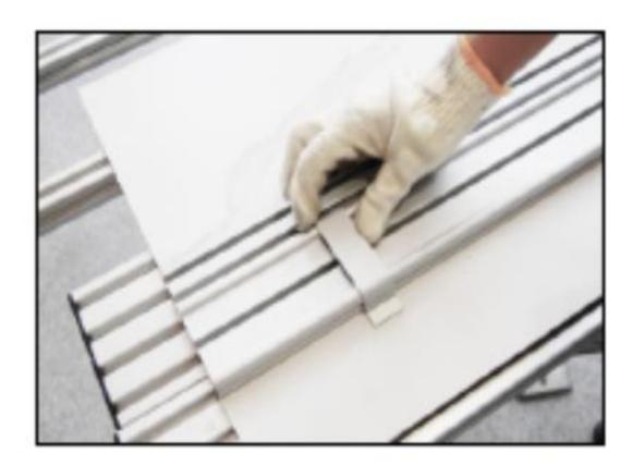
Mark the position where you want to cut. Align the edges of the gauge to the position.
