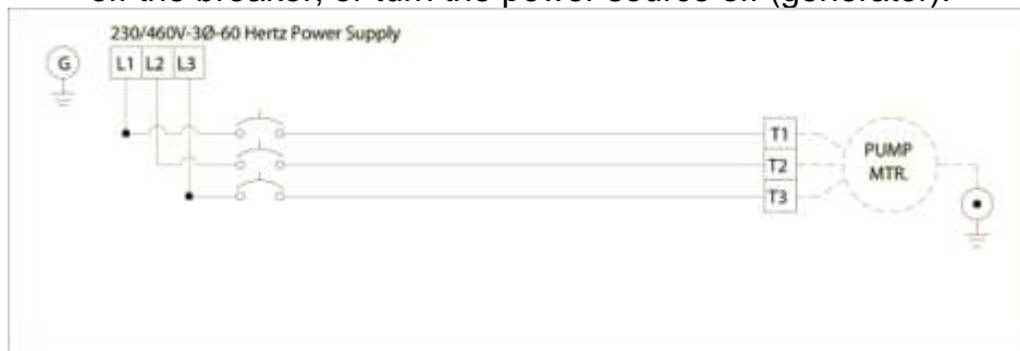
Typical 3 phase manual control 1
