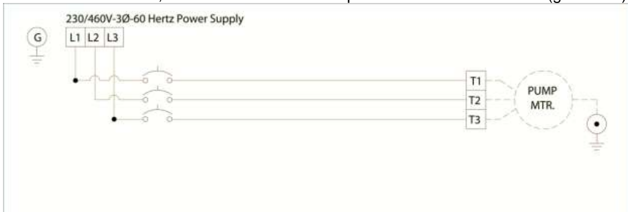
Typical 3 phase manual control 1
