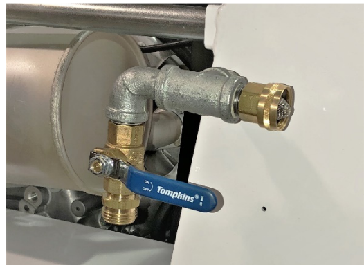
Water Valve on Left Side of Saw with Water Source Connection
