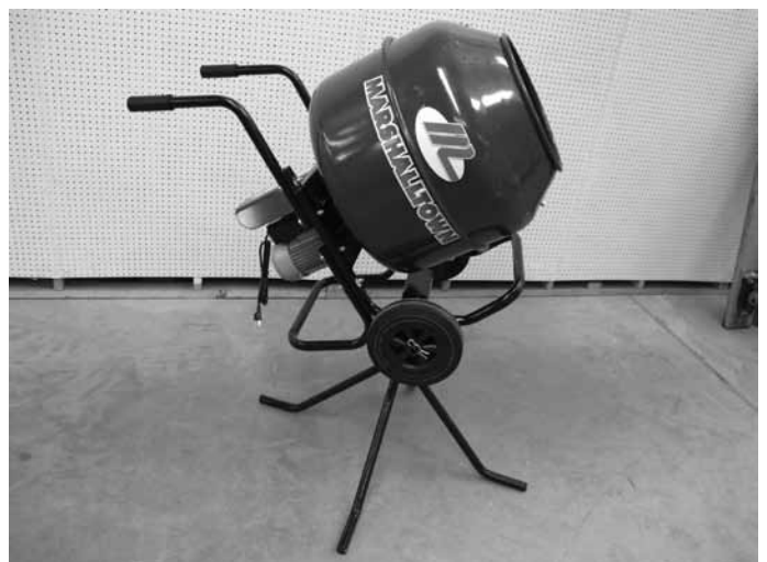
Completed mixer with pedestal.
