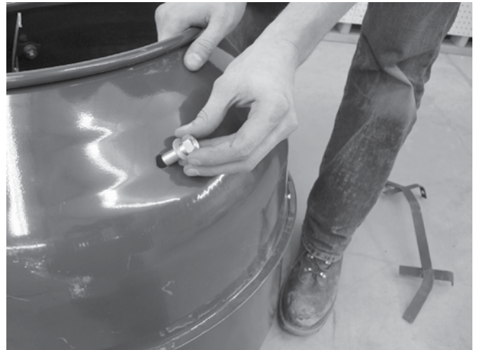
Insert bolts through drum.
