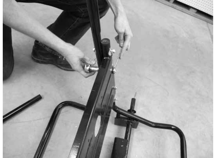
Fasten using a 14mm wrench and 14mm socket.
