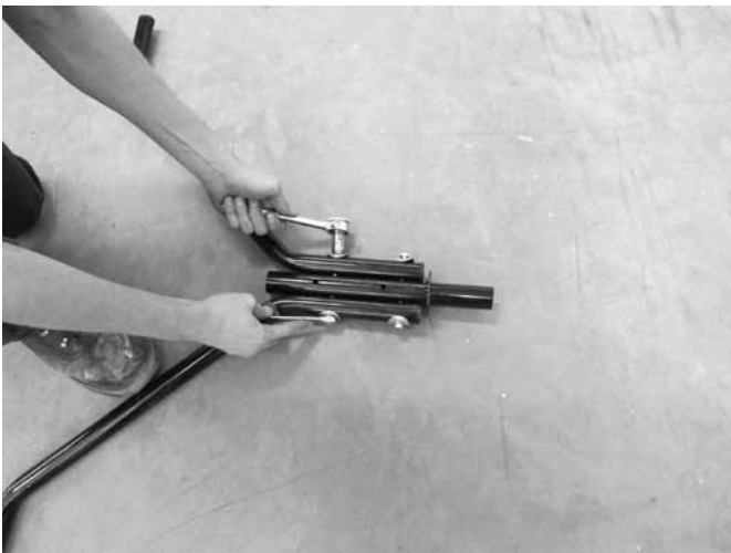
Tighten hardware using a 14mm wrench and 14mm socket.
