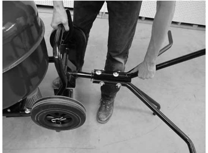
Lift mixer slightly and insert pedestal.
