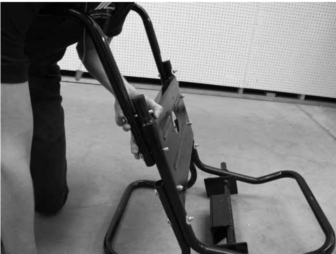
Use hardware 2B on top, 2A on bottom.
