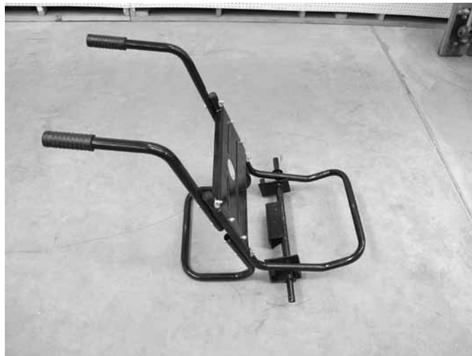
Finished frame with handles.
