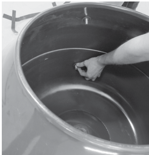
Place rubber washers onto bolts.
