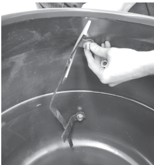
Install paddles with short side facing outward, towards top of the drum.
