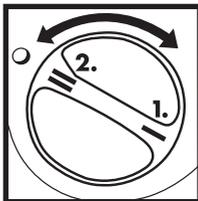
To change from one gear to the other, turn the gear selection lever through 180°.
