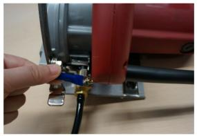
■ Turn the water valve to the position to stop the water flow.
