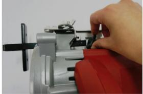
Adjust the parallel guide to the desired width from the blade, then tighten the retaining screw.
