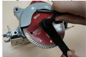
■ Finally, use the socket wrench to tighten the spindle bolt in a
