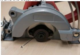
Inner flange (A) remains on the spindle.
