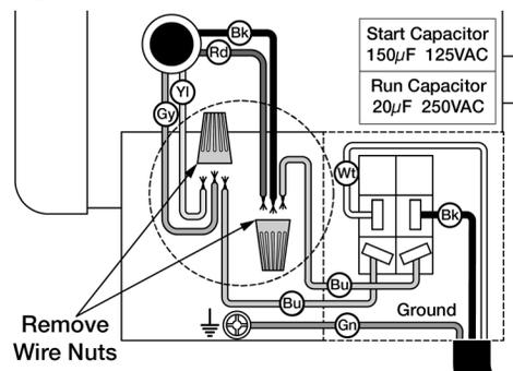
4. Remove the wire nuts. Replace the plug on the existing power cord with a NEMA 6-15 plug. The plug must be plugged into a matching outlet that is properly installed and grounded in accordance with all local codes and ordinances.
