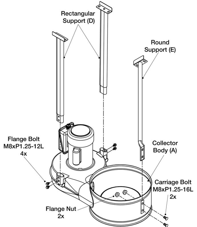
5. See Figure 5. Place Collector Body assembly on its side.
