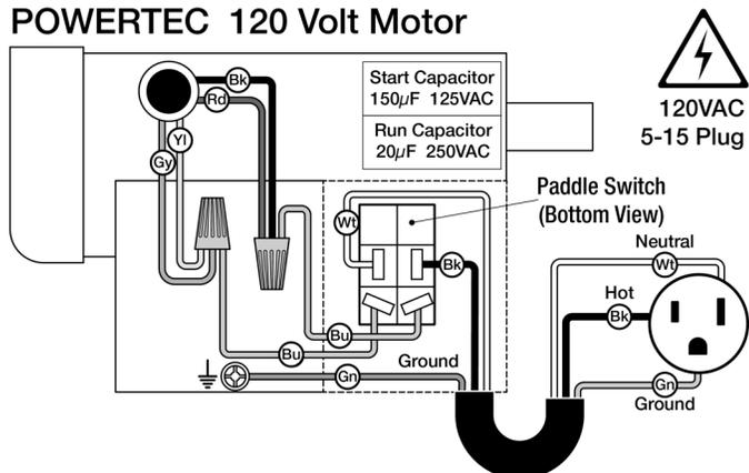
The permanently split capacitor motor has the following specifications:
