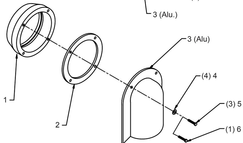
**PARTS LISTING - ILLUSTRATION #9 : 50mm INLET ASSEMBLY**
