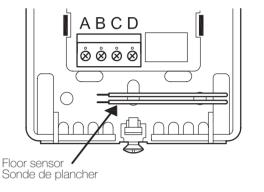
Thread the floor sensor cable through the hole in the power base. Push the electrical wires to the back of the electrical box.
