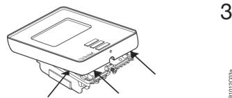
Loosen the screw at the bottom and remove the faceplate. Do not attempt to remove the screw completely.
