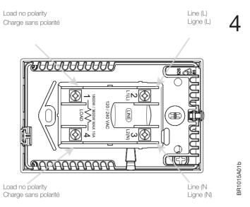
Turn power source OFF at breaker panel. Connect power supply wires to line side and heating cable wiring to load side of power base.
