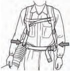
Place the hip strap over the hip and not too far down on the stomach. Tighten the hip strap so that you feel the weight of the blower resting on your hip. Tighten and adjust the breast belt for the best working position.
