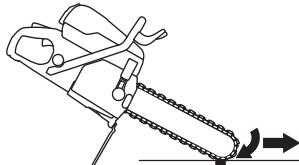
Never move the machine when the cutting equipment is rotating. Gyroscopic forces can obstruct the intended movement.
