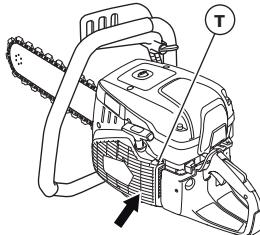
Rec. idle speed: 2700 rpm
