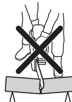
If the chain is pinched or stalled in the kickback zone, the reactive force will push the power cutter up and back towards the user in a rotating motion causing serious or even fatal injury. Be alert for potential movement of the work piece. Be alert to movement of the work piece or anything else that can occur, which could cause the cut to close and pinch the cutting equipment.
