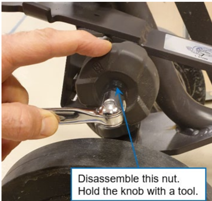
Figure 5: Disassemble the nut holding the knob.
