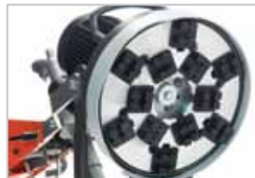
Durable, steel constructed diamond disc holder has a low-profile with recessed locking mechanism. This reduces overall height of tooling, keeping the machine closer to the ground.
