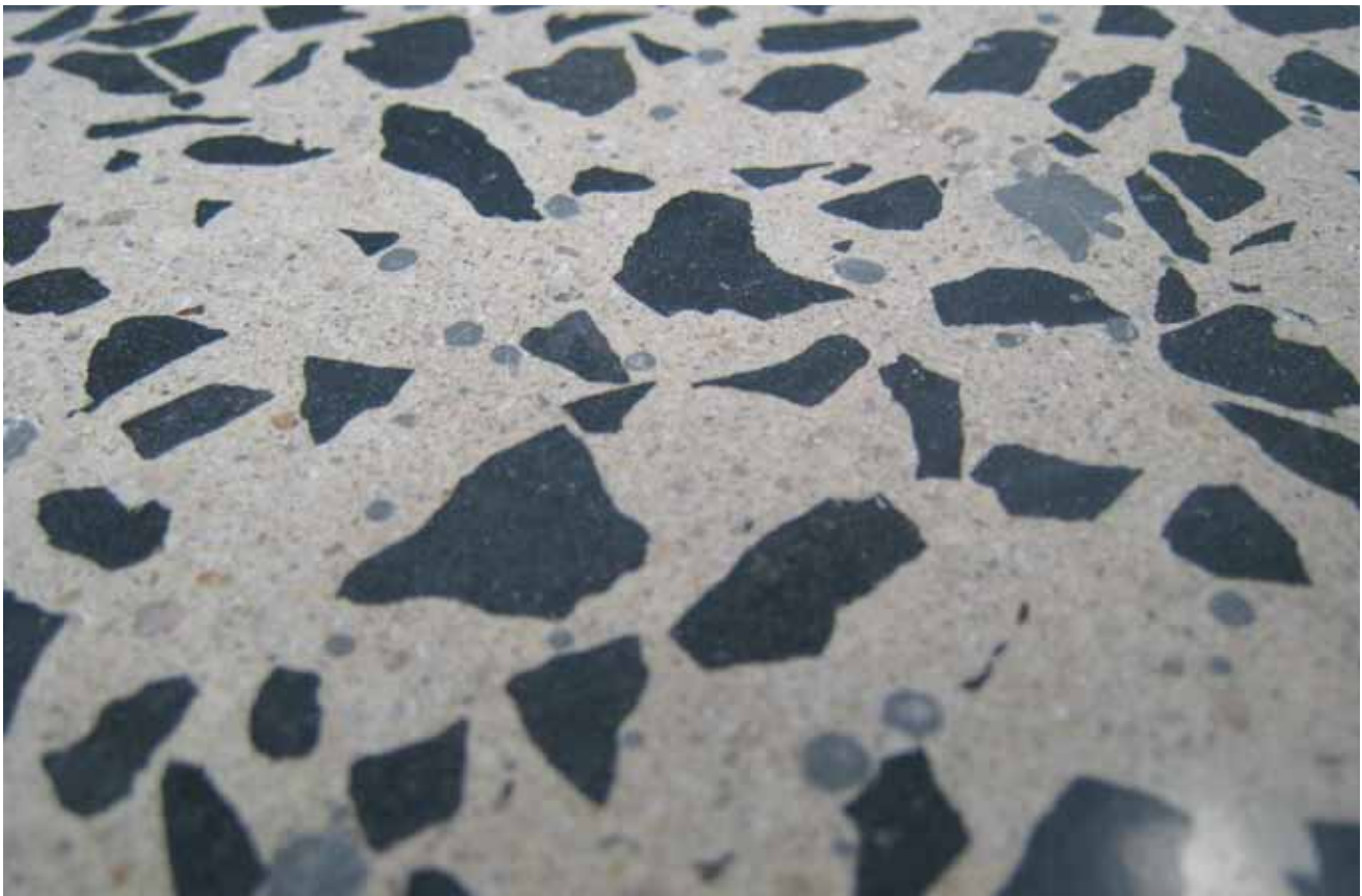
Holes filled when grinding with 120 grit metal-bonded diamonds and GM 3000™.
