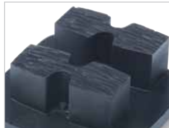
Husqvarna segment shape has more active diamonds than a basic rectangular shape. This means more aggressive grinding. They are pre-sharpened, enabling them to work with 100% efficiency at the start, without the need to dress the tool.
