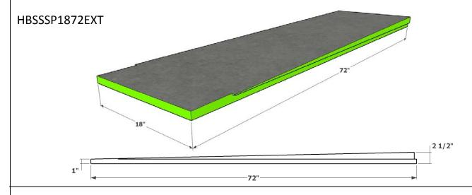
\*Side extensions are pre-notched for extending either side of any standard single slope pan for use with line drain\*
