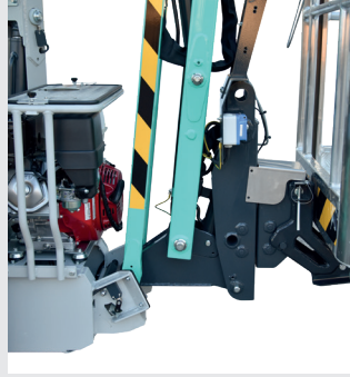
Compactness of the jib assembly hosting the load cell and basket quick mounting system
