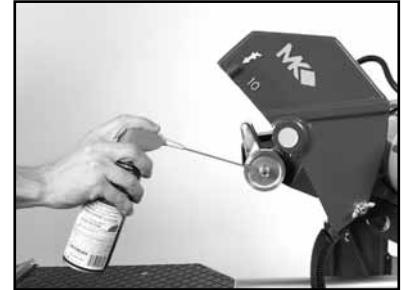
(C) Lubricate the Arbor Shaft.
