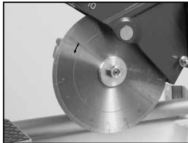
(B) Check for proper blade rotation.
