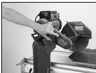
(A) Loosen Cutting Head Adjusting Knob.
