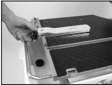
(A) Remove the Adjustable Cutting Guide.
