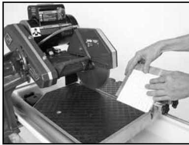
(B) Position the tile on the 45° Bullnose Miter Guide and the Ruler/Stop. Turn the motor ON.
