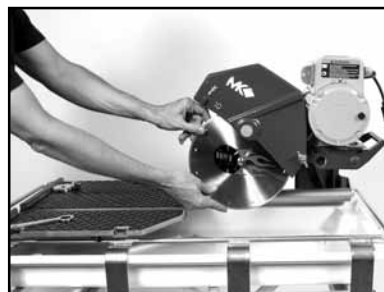
(E) Install Diamond Blade onto Blade Shaft.
