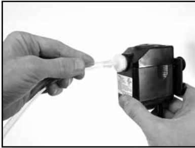
(D) Remove the Cooling Transfer Tube and check for flow. If flow exists, refer to water pump manual.
