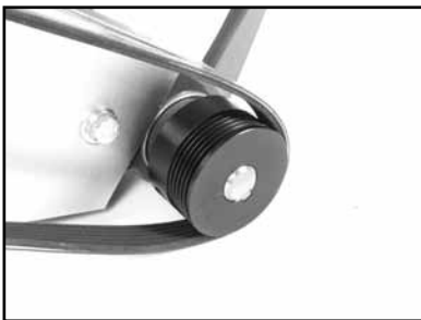
(M) Verify the Micro-V Belt is seated in the grooves of both pulleys
