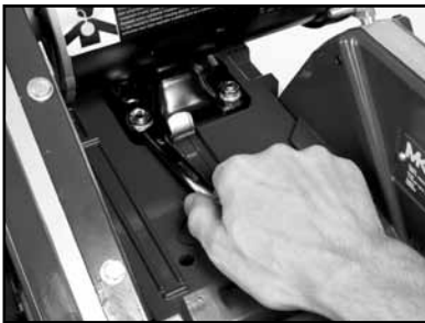
(P) Tighten the four motor mounting bolts
