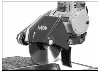
(B) Inspect Diamond Blade for damage.
