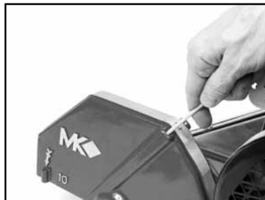
(G) Rod the Cooling Channels and then recheck flow.
