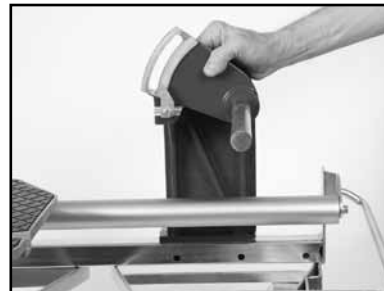
(E) Remove and relocate the Post to the rear Post retaining holes.
