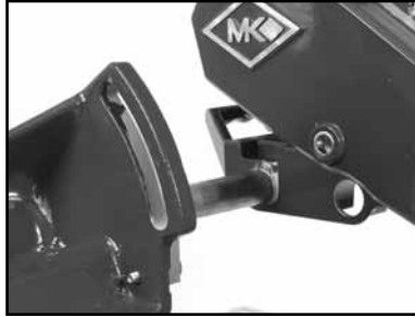
(B) Align Cutting Head rear Pivot Hole to the Post Pivot Shaft and slide onto shaft.
