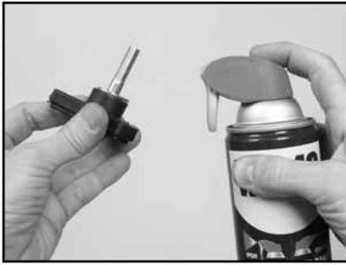
(J) Lubricate the Cutting Head Adjustment Knob.
