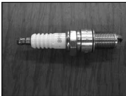
(A) Replace Spark Plug. Refer to Engine Manual for details.
