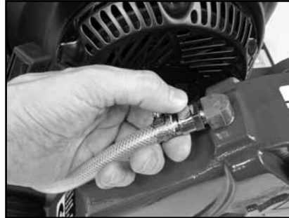
(B) Remove the Cooling Transfer Hose from the Blade Guard by pressing the quick release.
