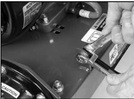
(M) Verify the stop Clip is installed as shown.
