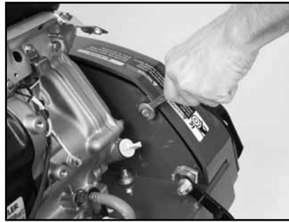
(B) Locate and remove the Belt Guard Retaining Bolts and then remove the Belt Guard.
