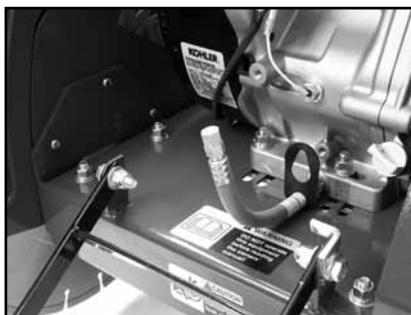
(A) Change engine oil every 100 hours. Refer to Engine Manual for details.
