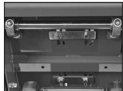
(C) Lubricate the Blade Shaft Bearings (Monthly).
