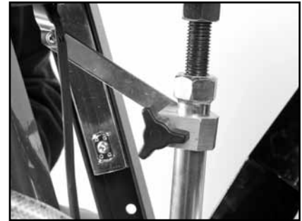
(C) Lubricate the Grease Fitting.
