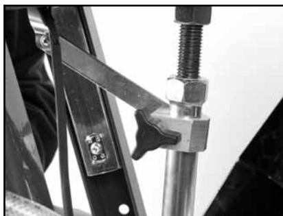
(B) Lubricate the Depth Control Screw (Monthly).
