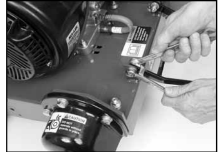
(L) Install the Pointer on the opposite side, next to Blade Guard.
