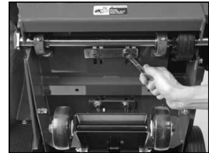
(F) Locate the four lower Engine Mounting Bolts on both ends of the motor and loosen.
