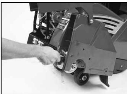
(G) Install the Blade Guard on the opposite side of the saw.
