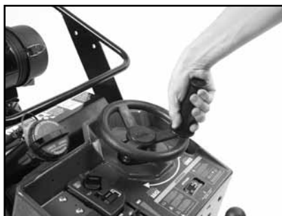
(K) When the cut is complete, raise the Blade completely out of the cut by turning Depth Control Wheel counter-clockwise.
