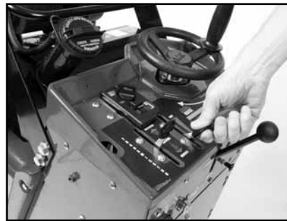
(B) Move the Throttle Lever to lower blade speed. Place Fuel Valve in the OFF position.
