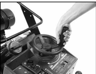
(J) Slowly lower the Blade until the desired level is reached and begin the cut.
