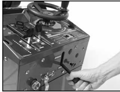
(E) Verify Neutral Engagement Handle is down, in Neutral. Choke engine as required for cold starting.
