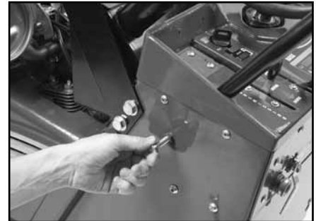
(C) Install one Washer onto each bolt. Install bolt through the Handlebar and into the holes and tighten.
