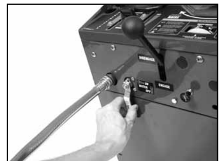
(L) Close Cooling Supply Valve.
