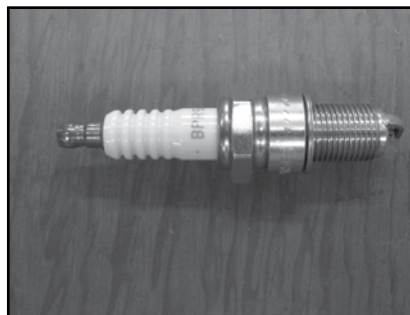
(D) Clean Spark Plug Weekly and re-adjust Spark Plug monthly. Refer to Engine Manual for details.
