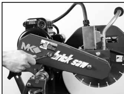
(G) Install the Belt Guard.
