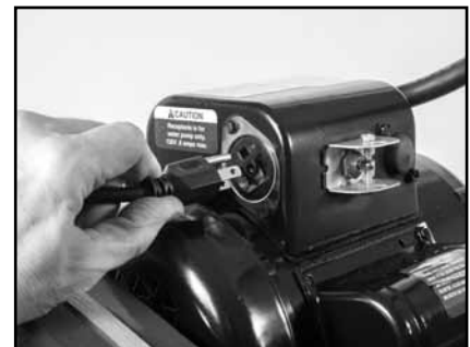
(C) Connect the Water Pump power cord to the receptacle found on motor.
