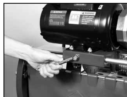
(F) Tighten the Motor Adjustment Strap using a 9/16-inch wrench to remove slack.
