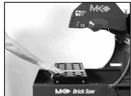
(C) Verify movable Cutting Table is seated correctly by moving table back and forth
