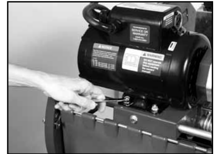
(C) Clean the remainder of the MK-2000. Verify all Motor Mounting Bolts are tight.
