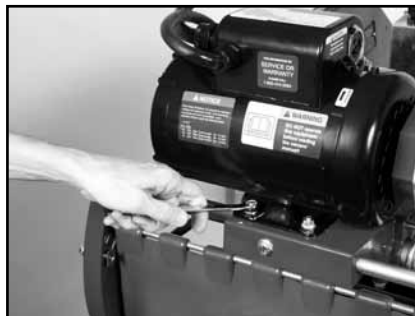
(B) Loosen the Motor Mounting Bolts using a 1/2 inch wrench; if retensioning only go to step F.
