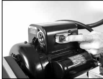
(B) Move the Voltage Change Switch to the desired voltage setting.
