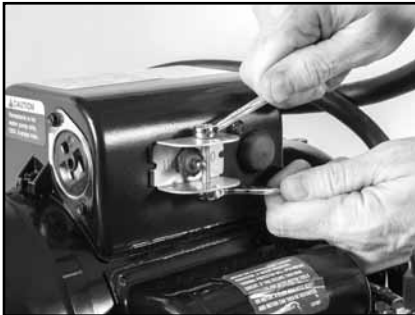
(A) Remove the Voltage Change Switch locking nut and bolt using 3/8" and 5/16" wrenches.
