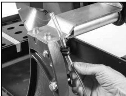
(A) Insert cooling transfer hose through loop.
