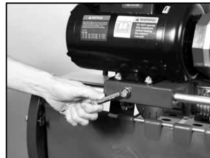
(C) Loosen the Motor Adjustment Strap using a 9/16-inch wrench.
