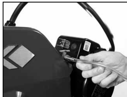
(B) Connect the Cooling Transfer Tube to the inlet connection of the Blade Guard.
