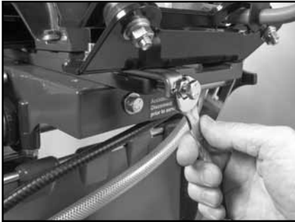
(P) Verify the Engine Adjustment Strap Lock-Nut is loose then tighten the Adjustment Strap.
