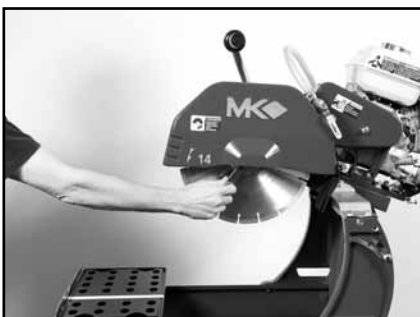
(Y) Install the Diamond Blade.
