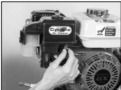
(D) Move the Throttle Lever to adjust blade speed. Refer to Engine Manual for your specific engine.
