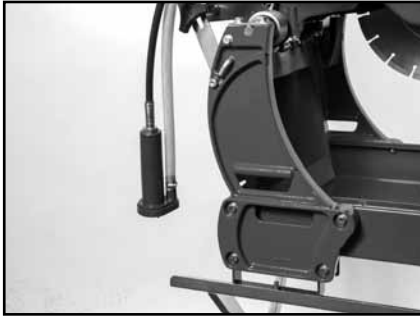
(A) Move Water Pump Assembly to the outside of the Water Basin.
