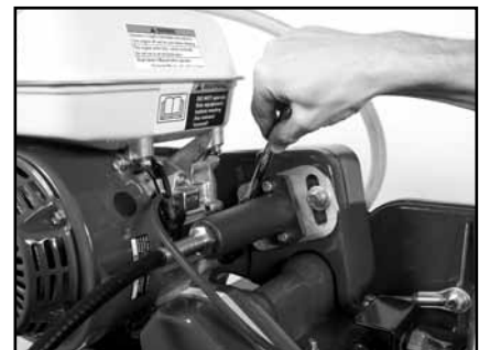
(C) Loosen Water Pump Drive end Pivot Plate front and rear Retaining Bolts.
