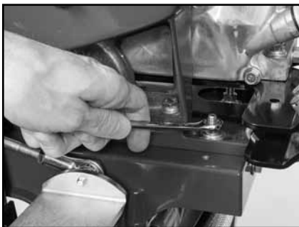
(D) Loosen engine mounting plate. If re-tensioning, go to Step J. 5 bolts, 4 under motor, 1 to left of power switch.
