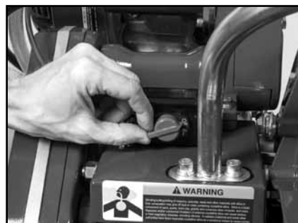
(B) Place Engine Switch in the OFF position. Refer to Engine Manual for complete shut down procedure.
