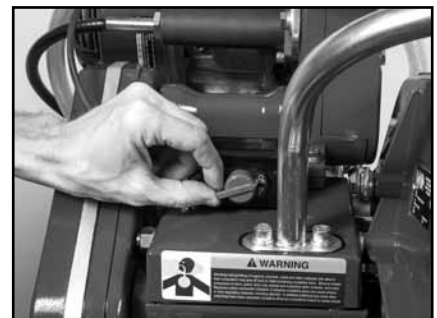
(C) Place Engine Switch in the OFF position. Turn OFF saw. Refer to Engine manual for complete shut down procedure.
