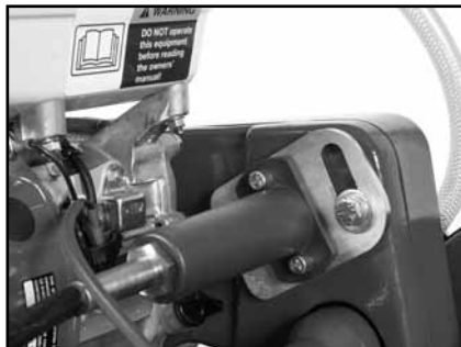
(D) Loosen Water Pump Drive End Pivot Plate front and rear retaining bolts.
