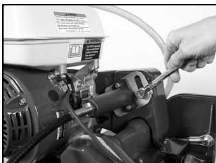
(D) Pivot front of Water Pump drive end Pivot Plate up and tighten the Retaining Bolts.
