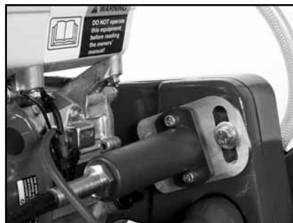
(B) Identify the Water Pump Pivot Plate.
