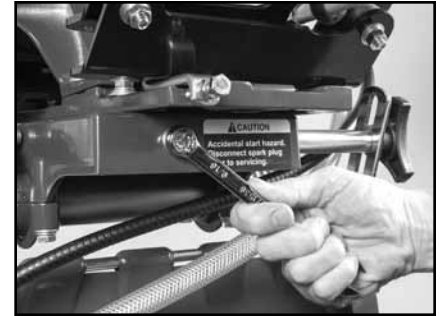
(R) Continue adjusting Micro-V Belt until tension is correct then tighten the Engine Adjustment Strap Lock-Nut.
