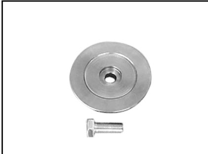
(A) Remove and clean Diamond Blade Outer Flange and Retaining Bolt.
