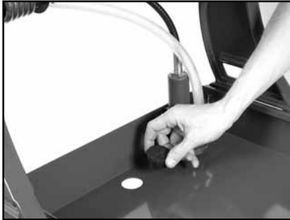
(A) Remove the Drain Plug and place a catch basin below the drain hole.
