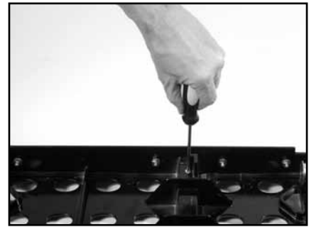
(C) Remove the two Protective Wooden Strip Retaining Screws.
