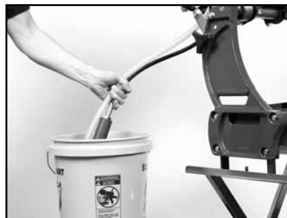
(B) Place Water Pump in a container of clean water. Run MK-2000 Gas Saw until clear water is seen at blade cooling ports (Approx. 1 minute).
