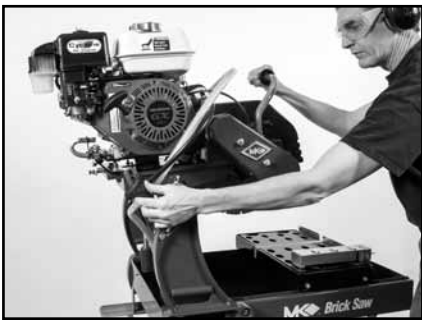
(J) Raise Cutting Head and lock into place. Refer to Engine Manual for complete shutdown procedure.
