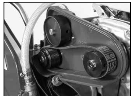
(O) Verify the Micro-V Belt is seated in the grooves of both pulleys.
