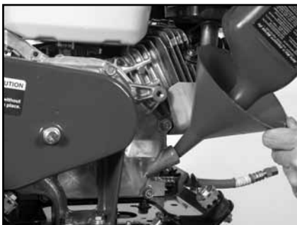
(A) Change engine oil. Refer to Engine Manual for all required engine maintenance.
