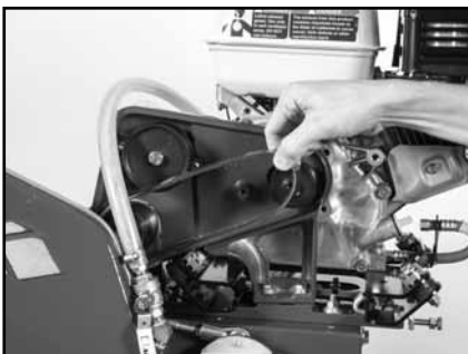
(M) Remove the Micro-V Belt.
