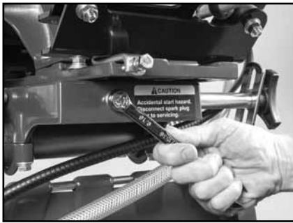
(J) Verify the Engine Adjustment Strap Lock-Nut is loose then tighten the Adjustment Strap.
