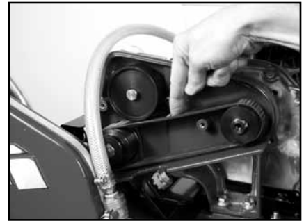
(I) Check Belt for proper tension. If tension correct, go to Step U (proper tension 1/8-inch).
