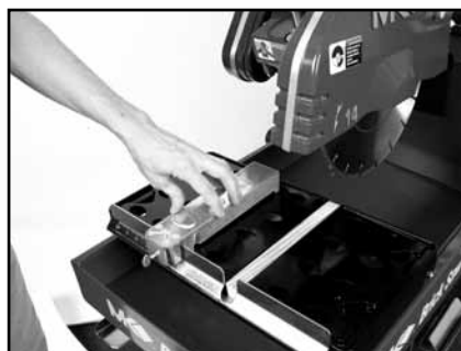
(B) Position adjustable Cutting Guide above movable Cutting Table. Align parallel slots. Seat and tighten the adjustable Cutting Guide retaining thumbscrew.
