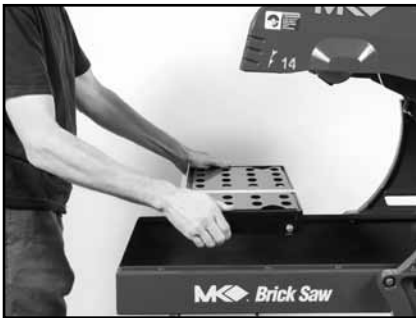
(A) While holding the front, position movable Cutting Table roller wheels above Guide Rails
