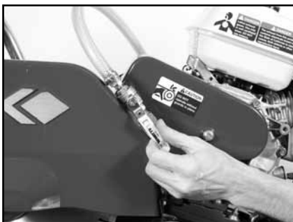
(D) Open the Cooling Flow Control Valve and adjust flow. Verify cooling flow exists on both sides of the blade.
