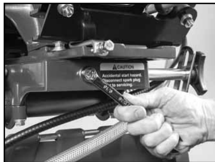
(E) Loosen Engine Adjustment Strap Lock-Nut then loosen the Engine Adjustment Strap.
