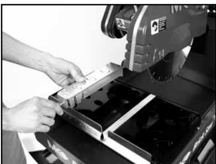
(A) Loosen adjustable Cutting Guide retaining thumbscrews by turning counter-clockwise.
