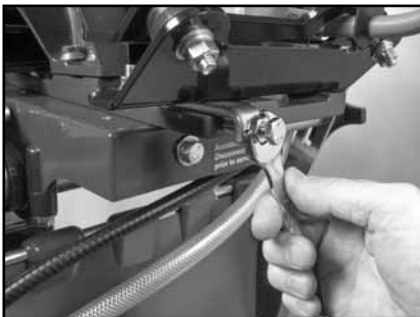
(S) Tighten the Strap Lock-Nut.
