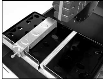
(B) Inspect Wooden Strip for excessive grooves.
