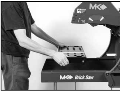
(A) Remove the movable Cutting Table.
