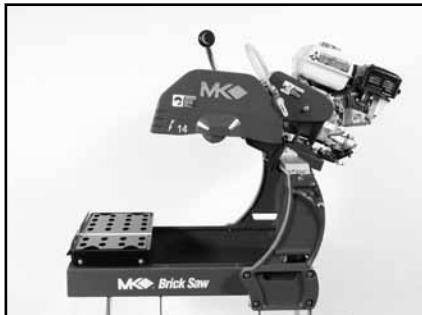
(A) Raise Cutting Head by loosening Cutting Head Lock
