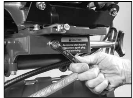
(L) Continue adjusting Micro-V Belt until tension is correct. Then tighten the Engine Adjustment Strap Lock-Nut.
