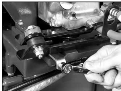
(K) Loosen Ending Adjustment Strap Lock-nut then loosen the Engine Adjustment Strap.
