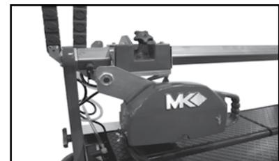
**NOTE:** The Cutting Head end will be heavier than the opposite end. Add block or packing material under Cutting Head (as shipped) for transporting via vehicle.
