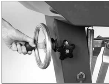
(B) Raise the Cutting Head by turning the Depth Control Wheel clockwise.
