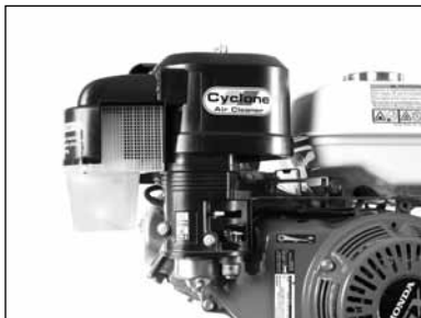
(A) Replace engine Air Filter. (See Engine Manual)
