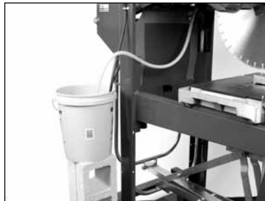
(E) Attach the Cooling Valve to the Transfer Tube to verify flow – if no flow, replace valve.
