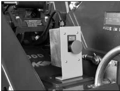
(E) Turn on Emergency Stop Switch.
