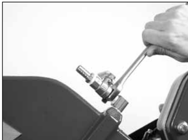
(D) Verify Cooling Valve operation by removing the valve from the Blade Guard.
