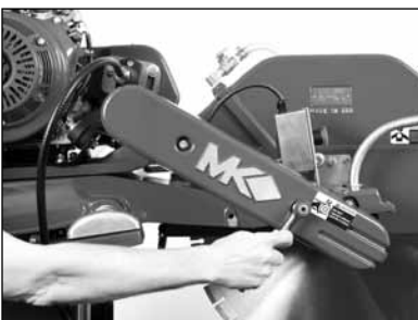
(A) Remove the Belt Guard Retaining Bolts.
