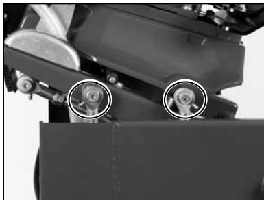
(D) Front and Rear Connecting Arms, right side lubrication points, if equipped.
