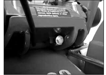
(I) Tighten the Engine Adjustment Strap Bolt to remove slack.
