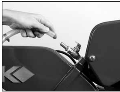
(B) Remove Transfer Tube from Blade Guard.
