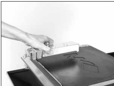
(A) Loosen the Thumbscrew. Align the Adjustable Cutting Guide above the Movable Cutting Table Ruler/Stop.
