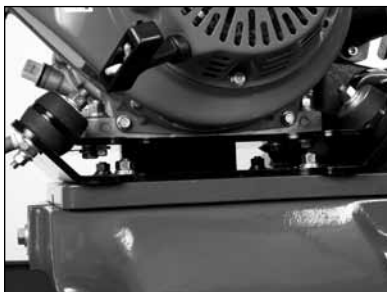
(D) Loosen the four engine bolts mounting plate. If re-tensioning, go to step I.
