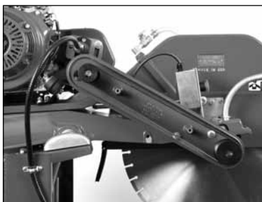
(B) Inspect the belt for cracks, fraying, separation and wear. Go to step D if replacement required.
