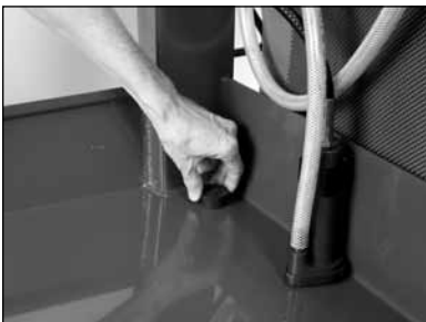
(A) Install the Drain Plug. Fill the water basin with clean water.
