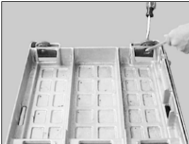
(A) Remove Roller Wheels. Rotate counter-clockwise to loosen.
