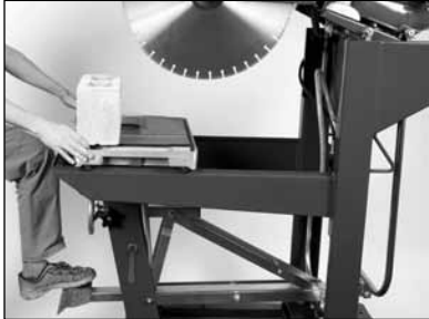
(A) Position masonry piece. Adjust the height of the Cutting Head as necessary, start engine.
