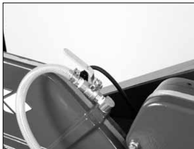
(B) Open the Cooling Flow Control Valve and adjust flow. Verify proper cooling flow on both sides of the blade.
