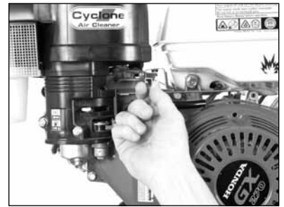
(C) Move the Throttle Lever to 1/3 open.
