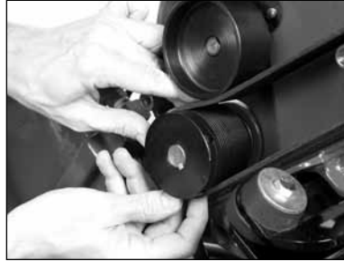
(H) Verify the belt is seated in the grooves of both pulleys.
