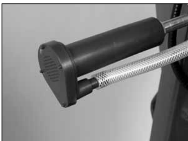
(A) Clean the Water Pump suction of all debris.
