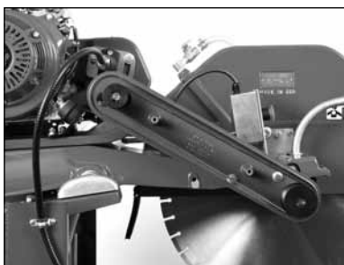
(B) Check belts. (See Belt Inspection, Adjustment and Replacement)
