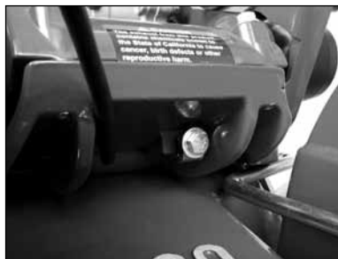
(E) Loosen Engine Adjustment Strap Bolt push the Engine Mounting Plate toward the front of the saw to loosen the belt.
