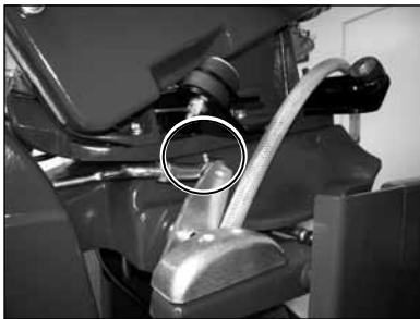
(A) Rear Blade Guard Stay-level pivot point lubrication point, if equipped.
