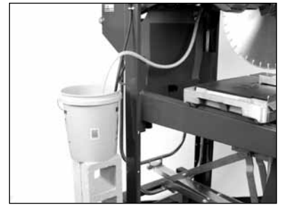
(C) Place Water Pump in clean water source and check for flow. (if no flow go to step G)
