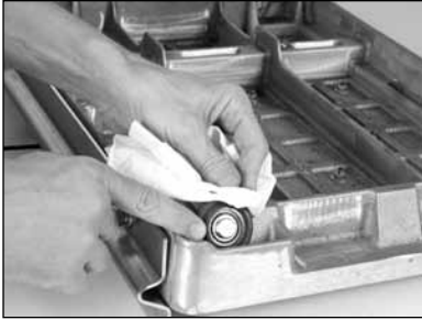
(D) Check Movable Cutting Table Roller Wheels for wear.
