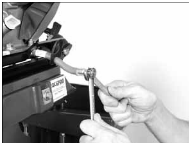
(A) Change engine oil. (See Engine Manual)
