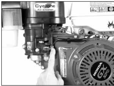
(A) Place Fuel Valve in the ON position.
