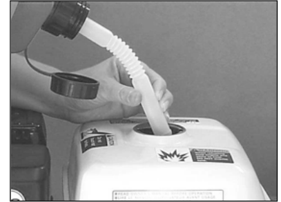
(C) Fill Fuel Tank until level is below throat.
