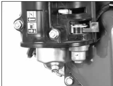
(B) Clean Fuel Sediment Cup. (See Engine Manual)
