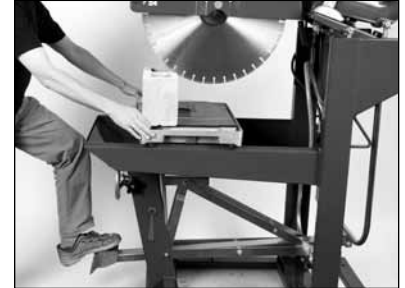
(C) Step Cut "Push" Stroke. Lower Cutting Head 1/4" -1/2" during Push Stroke.
