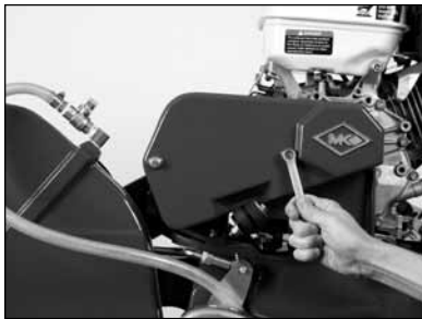
(A) Remove the Belt Guard Retaining Bolts.
