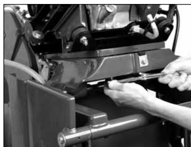
(K) Tighten Engine Mounting Plate.
