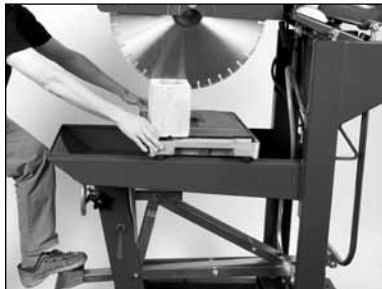
(E) Repeat Steps C and D until cut complete. Turn the saw off when work is complete.
