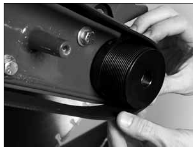
(H) Verify the belt is seated in the grooves of both pulleys.
