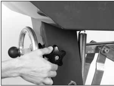
(A) Unlock Cutting Head.
