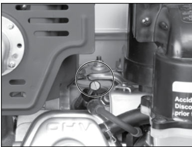
(D) Clean and readjust engine Spark Plug. (See Spark Plug Adjustment and Replacement)
