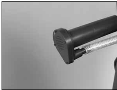
(H) Verify Water Pump suction is clean and pump impeller is turning. Pump Impeller is inside water inlet.
