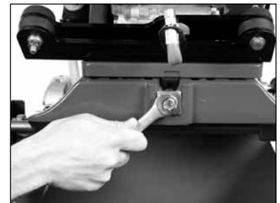
(I) Verify the Engine Adjustment Strap Lock-nut is loose then tighten the Adjustment Strap.
