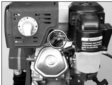
(B) Replace Spark Plug. (See Engine Manual)
