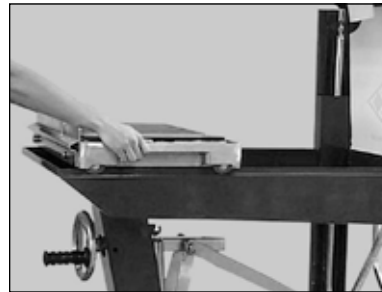
(E) Install Movable Cutting Table.
