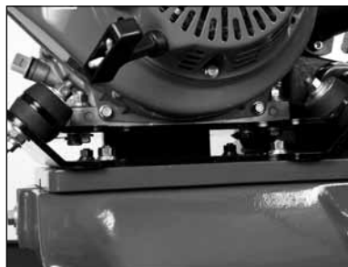
(B) Verify all Engine Mounting Bolts are tight.
