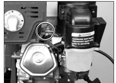
(C) Clean and readjust engine Spark Plug (See Engine Manual)
