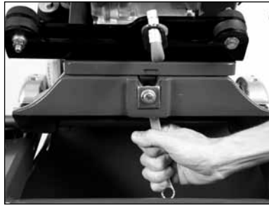
(E) Loosen Engine Adjustment Strap Lock-nut then loosen the Engine Adjustment Strap.
