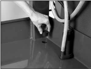
(A) Remove the Drain Plug.
