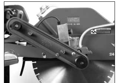
(C) Inspect belts. (See Belt Inspection, Adjustment and Replacement)
