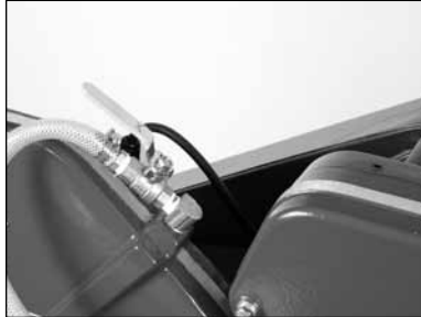
(B) Open the Cooling Flow Control Valve and adjust flow. Verify proper cooling flow on both sides of the blade.
