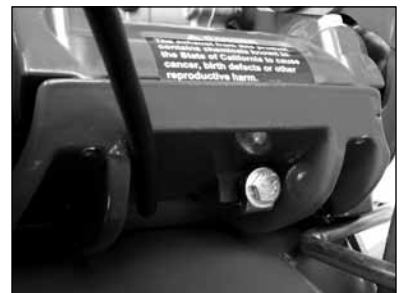
(C) Verify engine Adjustment Straps are tight.
