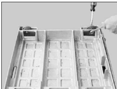
(D) Install Roller Wheel Retaining Nut and tighten. Rotate clockwise to tighten.
