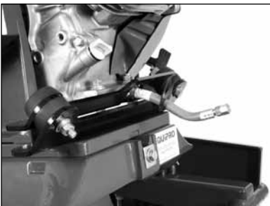
(A) Change engine oil after first month or first 20 operating hours. (See Engine Oil Change)
