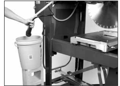
(C) Place the Water Pump Assembly into an external water source container. Fill the external water source container and place a catch basin below the Drain Hole.
