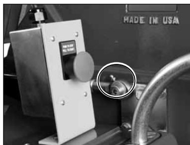
(B) Front Blade Guard Stay-level pivot point lubrication point, if equipped.
