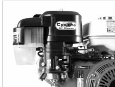
(H) Check Air Filter for cleanliness. (See Maintenance section if dirty)
