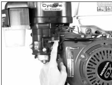
(H) Place Choke Lever in the OPEN position when engine is warm.
