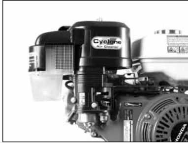
(E) Clean engine Air Filter. (See Engine Manual)
