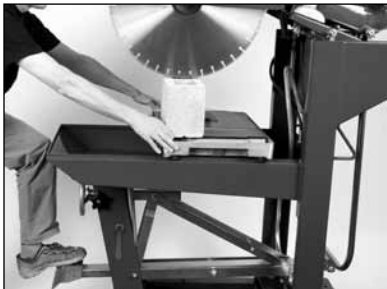
(D) Step Cut "Pull" Stroke. Lower Cutting Head 1/4" -1/2" during Pull Stroke.
