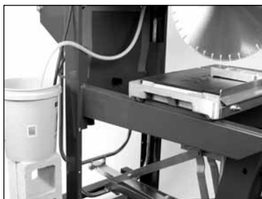
(B) Place the Water Pump in an external container of clean water. Run the saw until clear water is seen at the blade cooling ports (Approx. 1 minute).
