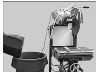
(C) Fill the external container until water completely covers the Water Pump intake
