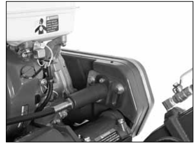
(I) Verify Water Pump drive end is in the operating position
