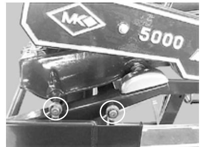
(C) Front and Rear Connecting Arms, left side (from front), lubrication points
