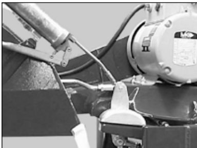
(G) Apply grease to the nine (9) Zerk Fittings of the MK-5005S (See Unit Lubrication page 29)
