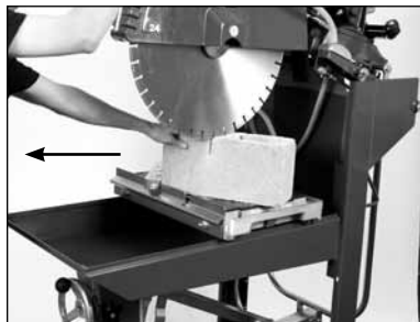
(E) Lower Cutting Head 1/4" -1/2" during "Pull" Stroke. Repeat Steps D and E until cut is complete. Turn the saw off when work is complete
