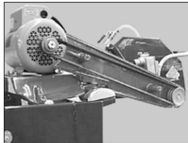
(E) Inspect the V-belt for cracks, fraying, separation and wear. Go to step G if replacement required
