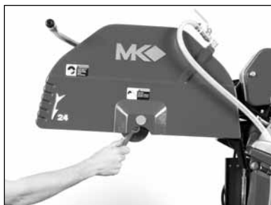
(A) Remove the Retaining Screw and Outer Flange with the blade wrench. Turn counter-clockwise to loosen
