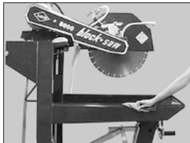
(H) Clean the movable Cutting Table Guide Rails
