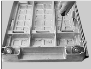
(E) Place movable Cutting Table on a work bench with the wheels up, and reinstall retaining screws
