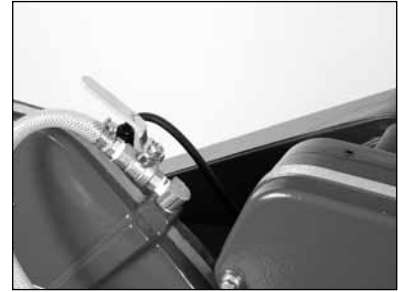
(C) Open the Cooling Flow Control Valve and adjust flow. Verify proper cooling flow on both sides of the blade
