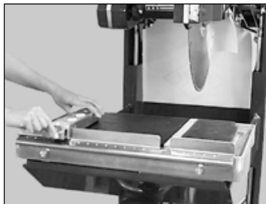
(A) Set edge of Cutting Guide to desired cut length on Ruler/Stop
