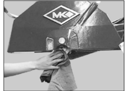
(C) Clean and lubricate the Inner Flange
