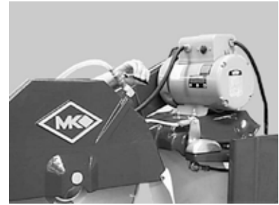
(C) Open the Coolant Flow Control Valve and adjust flow
