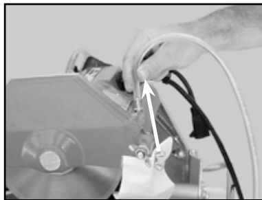
(B) Remove the Transfer Tube from the Blade Guard inlet, go to Step C
