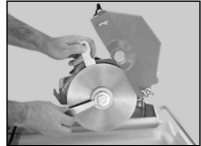
(F) Install the Retaining Nut and Outer Flange. Hold the Blade Shaft using the Inner Flange Retain- ing Wrench and tighten using the Blade Wrench
