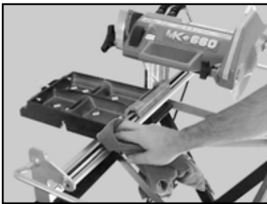
(J) Clean the movable Cutting Table Guide Bar
