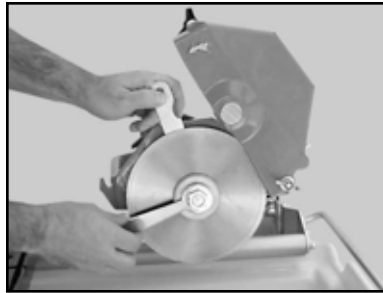
(B) Remove Retaining Nut and Outer Flange
