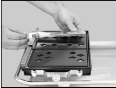
(A) Remove the adjustable Cutting Guide
