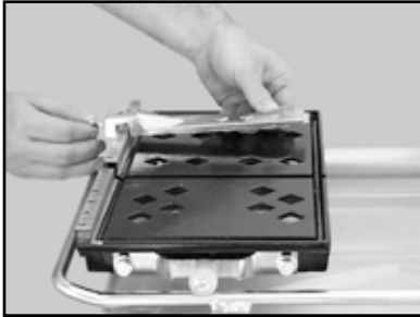
(A) Remove the adjustable Cutting Guide
