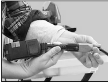
(B) Verify all plugs fully installed
