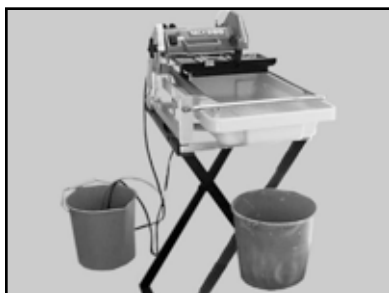
(A) Place an external catch Basin below the Water Pan drain hole
