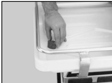
(A) Remove the Drain Plug
