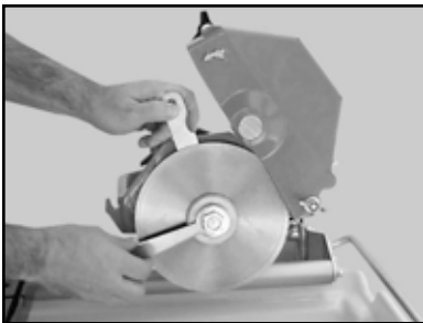
(A) Remove the Diamond Blade
