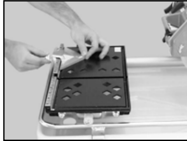
(B) Place the Dual 45° Flat Angle Guide on the Ruler/Stop
