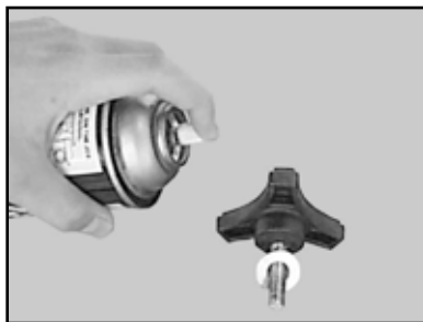
(M) Lubricate the Cutting Head Adjustment Knob
