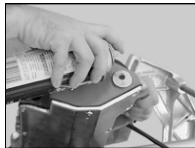
(N) Lubricate the Cutting Head Adjustment Knob retaining holes
