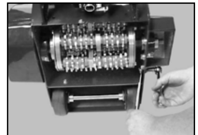
(R) Tighten the Shaft Guard Cover Retaining Bolts using 9/16 wrenches and/or sockets.
