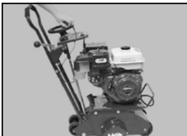
(A) Lower the Scarifier to its lowest position.
