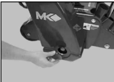
(P) Install the Shaft, Retaining Nut Cover onto the Belt Guard.
