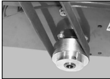
(N) Verify the V-belt is seated in all grooves of the Engine and Cutting Drum Pulleys.
