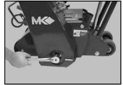
(L) Using a 15/16-inch socket tighten the Shaft, Inner Retaining Nut.
