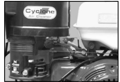
(F) Clean engine throttle linkage with a dry cloth.
