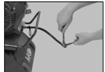
(C) Place a catch basin below the Oil Drain Line and remove the Drain Cap using two 1/2 –inch wrenches.
