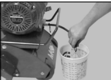
(D) Drain Oil the engine oil (conform to Federal, State and Local laws for disposal).
