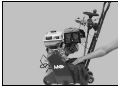
(E) Clean the remainder of the exterior surface of the scarifier (except the engine).
