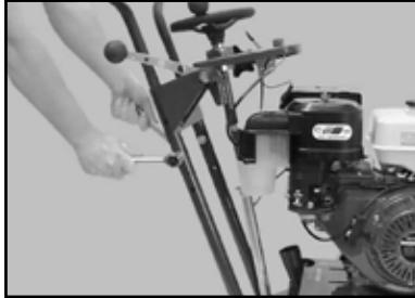
(B) Remove the Retaining Bolts using 9/16 wrenches and/or sockets.
