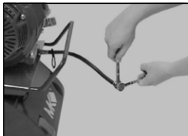
(E) Using two 1/2 – inch wrenches, install the Drain Cap onto the Oil Drain Line (Ensure the Cap is tight).
