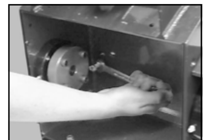
(I) Locate the V-belt Adjusting Screw Lock Nut inside the Cutting Drum Well. Loosen the nut using a 9/16-inch wrench.
