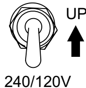
Figure 22. Full Power Switch 120V Position (Up)
