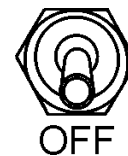
Figure 16. Manual-Off-On SW. (OFF Position)
