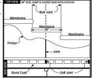
1/8" gap at all floor to wall transitions. Apply an acoustical sealant or sound perimeter tape at room perimeter. Soft joints in tile patterns are required as per TCNA Handbook method EJ171.
