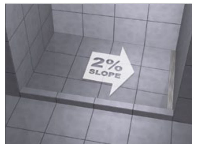
ProLine Drain at the side wall. Usually done when replacing a standard tub, because there is no need to move waste plumbing.
