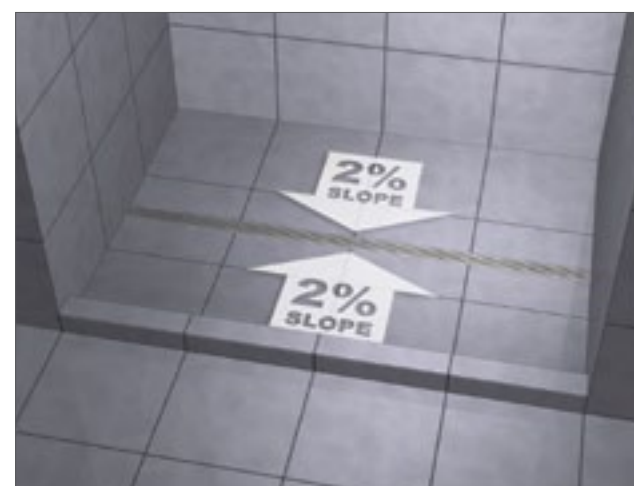
ProLine Drain at the shower center.
