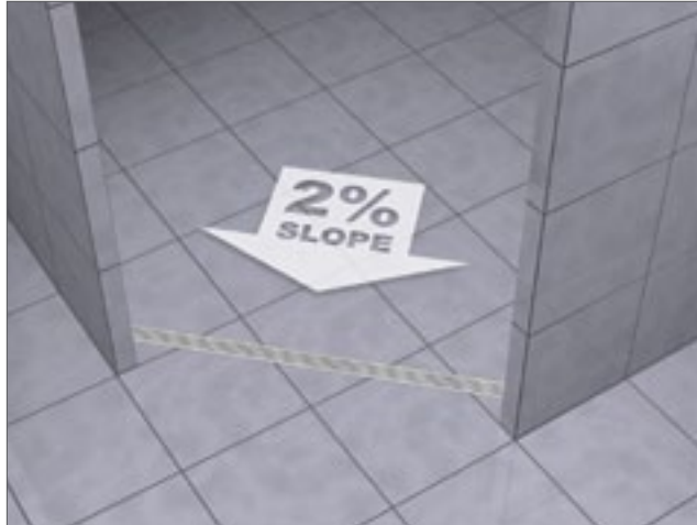
ProLine Drain at the entry opposite to the highest point.
