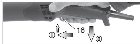
**Switching on:** Slide the trigger switch (16) forwards and then push the trigger switch (16) upwards.
