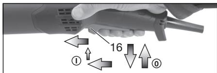
**Switching on:** Switch the machine on as described above. Now slide the trigger switch (16) forwards again and release in the front
