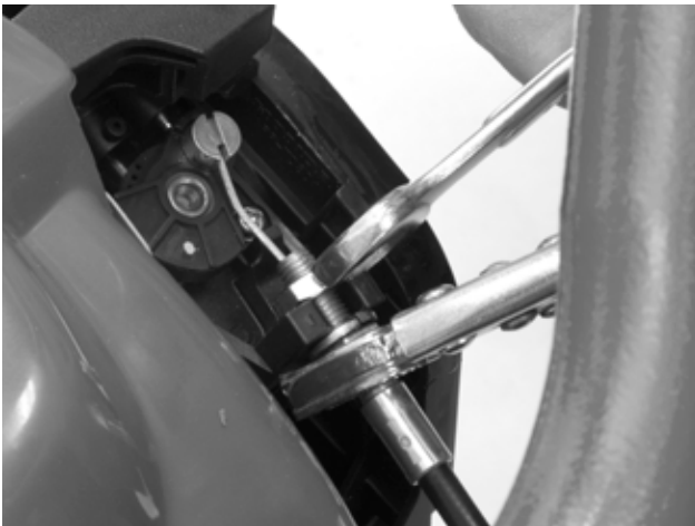
Step 3 – Fasten the throttle cable as shown. Make sure there is a nut on each side of plastic fitting. Make sure the cable does not work itself out of the plastic fitting while tightening.
