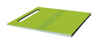
STL-TRAY is a pre-sloped shower tray for the channels in the Showertec Linear STL channel series. It is made of waterproof material and coated with a layer of embossed fiber-cement which increases resistance and allows a tight grip of tile glues. STL-TRAY is available in two widths (91 cm / 132 cm) and can be completed with extensions (see STL-EXT) and ramps (see STL-RAMP); the version with an increased thickness of 53 mm with raised panels (see STL-TRAY-R) is also available.
