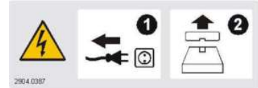
Warning electrical voltage risk of death! Always disconnect the mains plug from the power supply before opening the housing. 2904.0387
